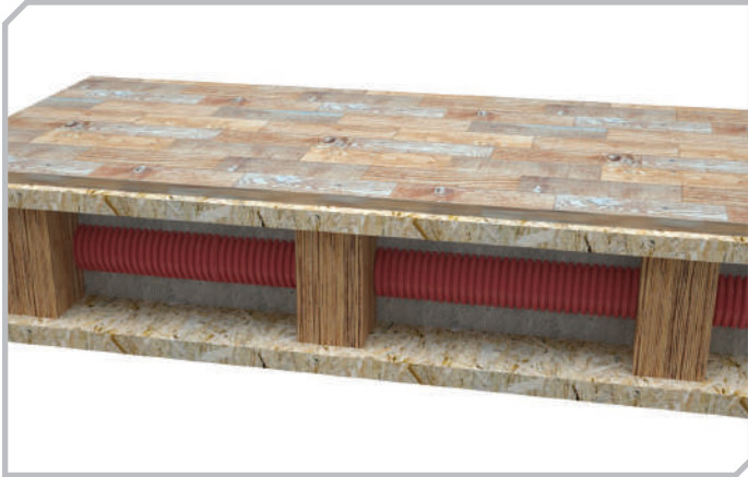
Inside wooden floor structures through the beams
